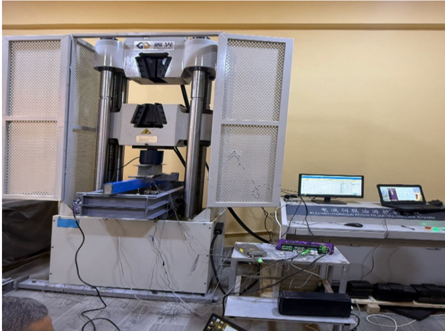
Figure 6. Compression Testing of Composite steel-concrete beam.
