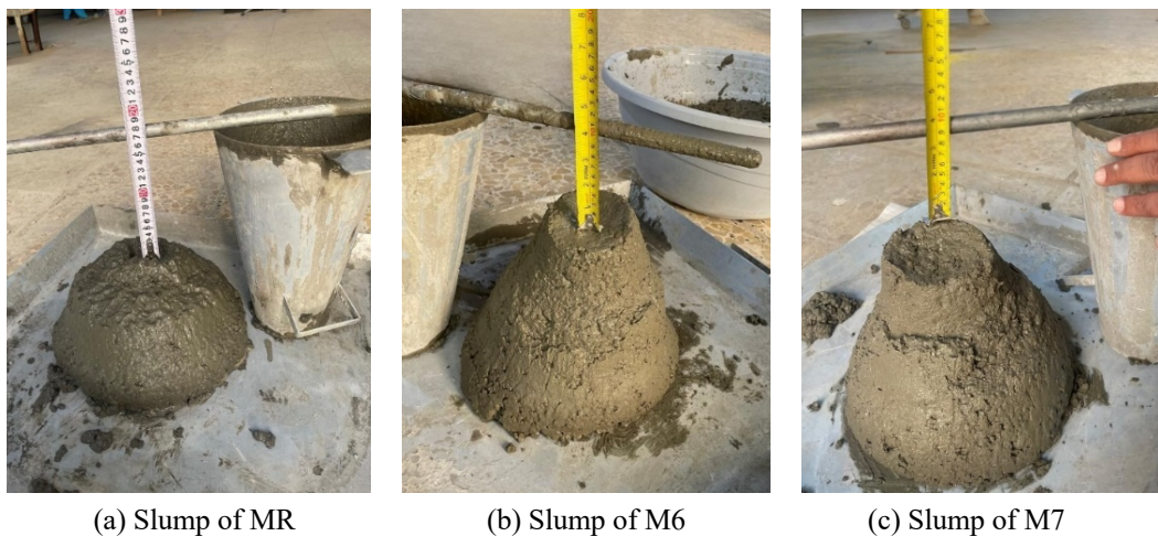
Figure 8. Measurement of mixtures' slump via the cone test
