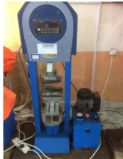
Figure 5. Matest apparatus for flexural strength tests
