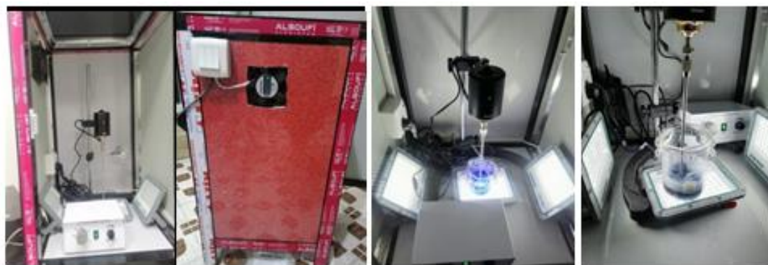
Figure 14. The batch reactor of the photocatalytic system to remove MB from synthetic wastewater using various types of catalysts.
