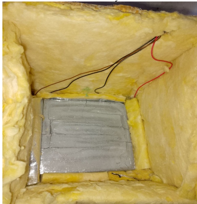
Figure 6. The ceramic material (CR2) is placed beneath the basin of the solar still.
