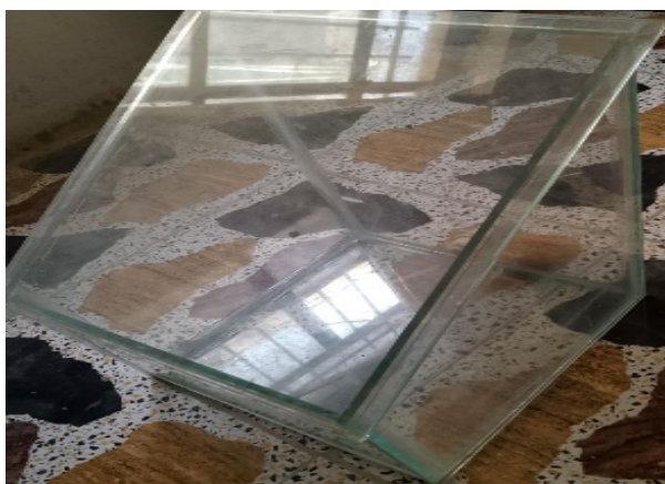
Figure 1. Single-slope glass solar still used in the experiments
