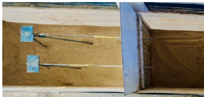
Figure 5. Batter Piles and Rods.
