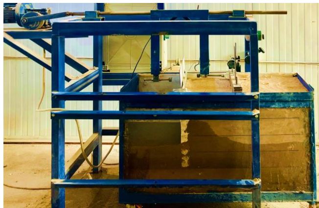
Figure 10. Installation of Anchored Sheet Pile Wall, Seepage Process after Prepared Soil.
