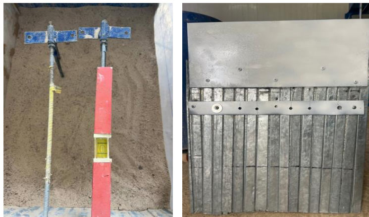
Figure 4. Anchored Sheet Pile Wall with Wale.
