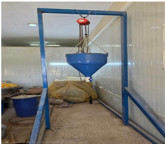
Figure 6. Sand Raining Device Used, [5].
