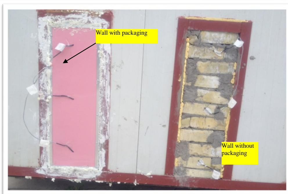
Fig.2.A brick wall with and without packaging
