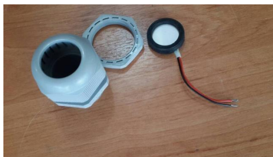
Figure 2. Picture of a sample of piezoelectric, plastic gland and washer.
