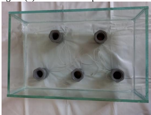
Figure 1. An image of a test vessel equipped with piezoelectrics.
