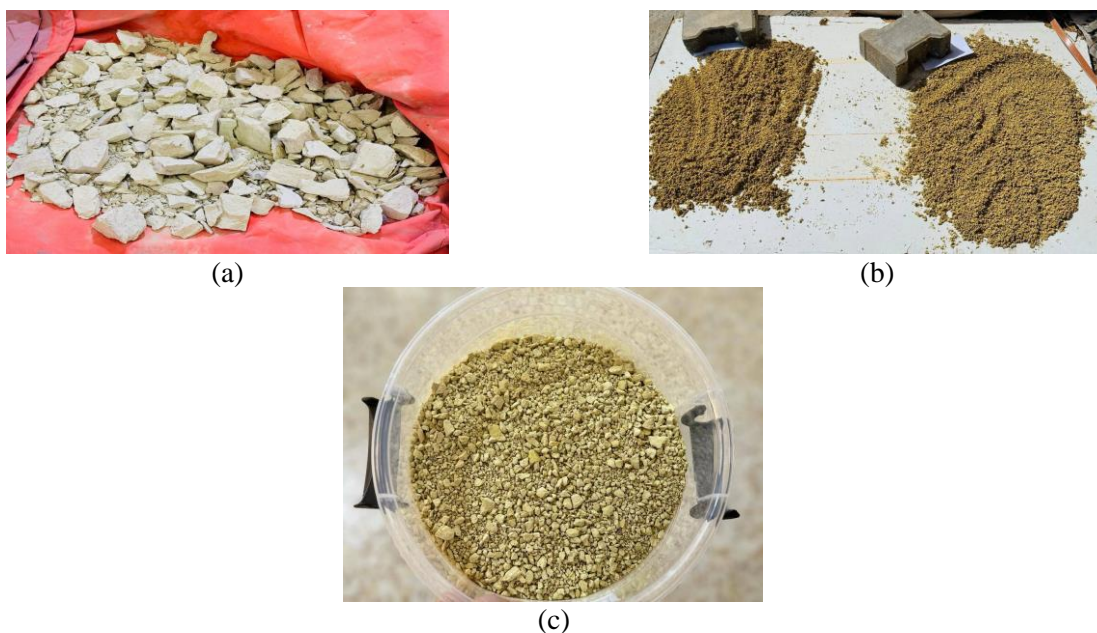
Figure 1. The preparation of Bricks, (a) At the beginning before drying, (b) After grinding and drying, and (c) The final adsorbent prepared after grinding and drying.
