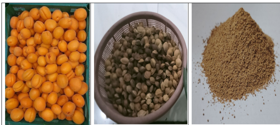
Figure 2. Preparation of Apricot Seed Powder with a Sieve of 600 Microns.
