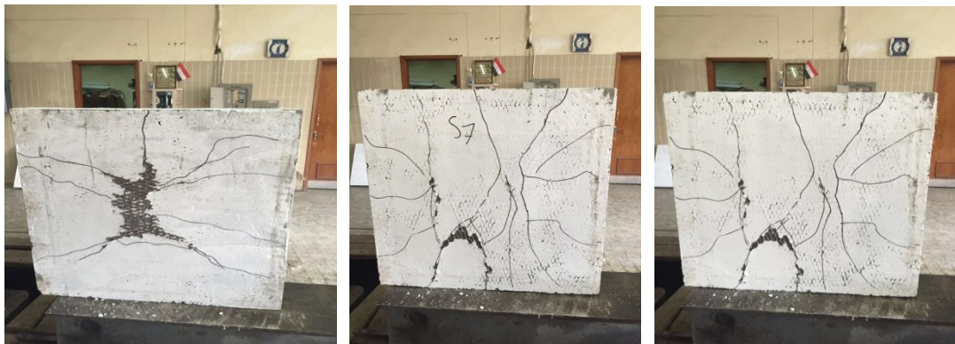
Fig 8: Cracks Pattern of Control Slab (A)
