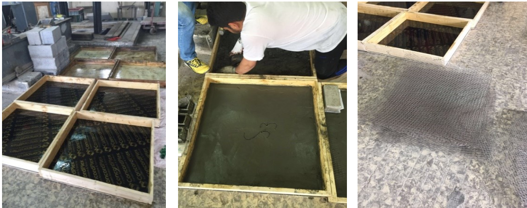
Fig 3: Placing the wire mesh and casting the slabs
