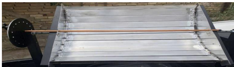
Figure 6. The Solar Collector Tubes.
