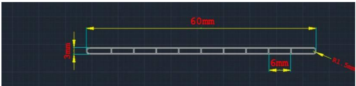
Figure 3.The Cross-Section of Aluminium Mini-Channel.
