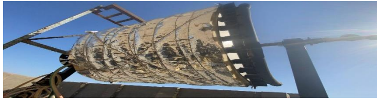
Figure 8. The Solar Collector with Fiberglass Insulation.
