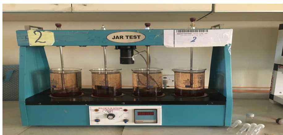
Figure 2. Maximum color removal of Congo Red using coagulants in Jar apparatus.
