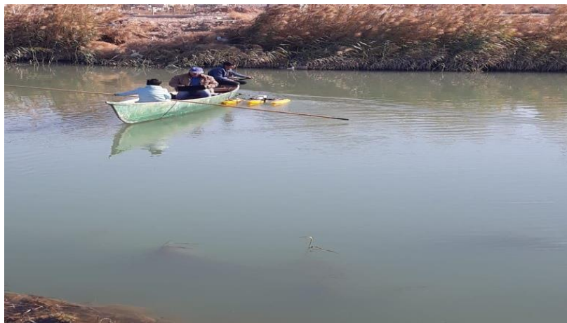
Figure 6 Measuring the discharge and velocity of each section along the channel using ADCP.
