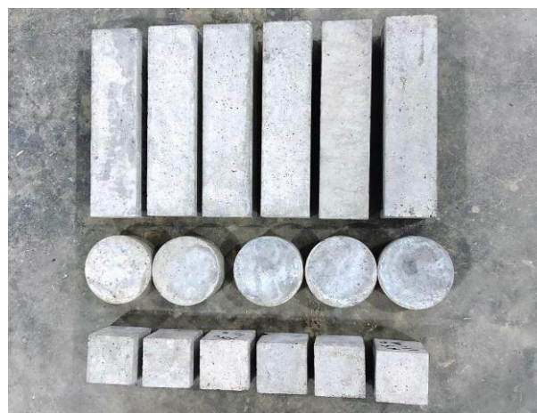
Figure 3 Cast specimens; beams, shallow cylinders and cubes
