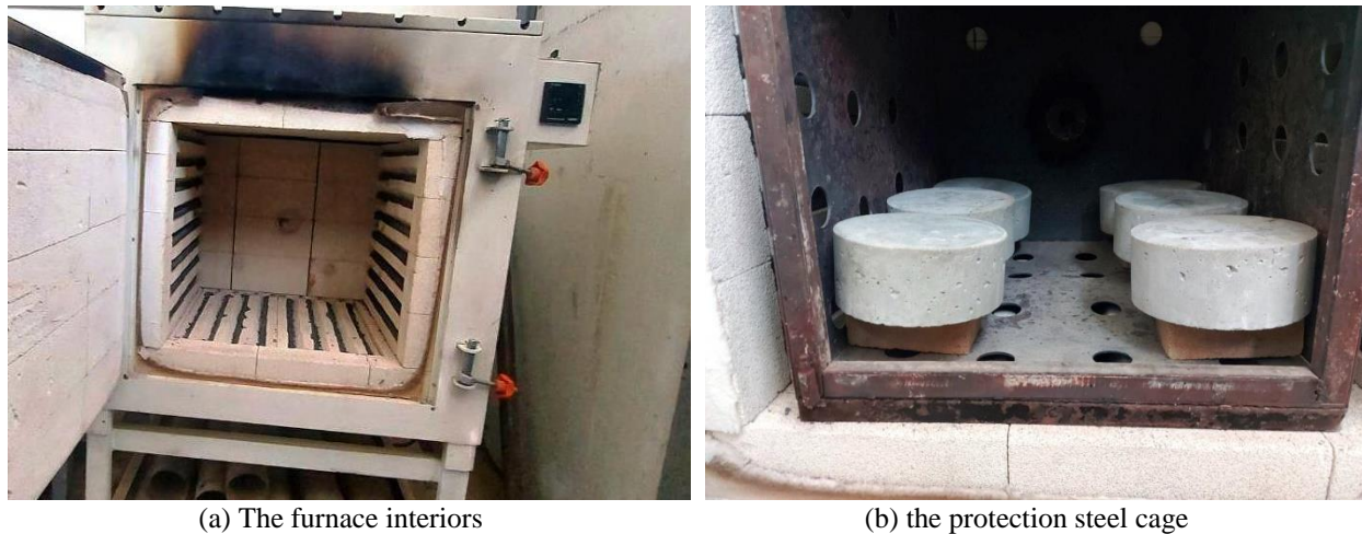
Figure 4 The used electrical furnace
