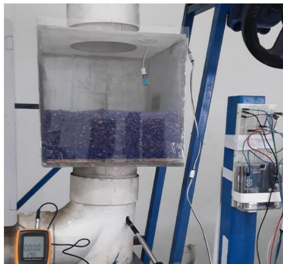
Fig.7: Places of the sensor & the way of recording the reading
