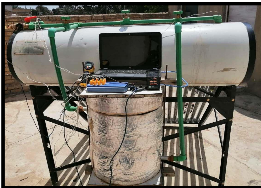
Figure 4 Solar water heater, Porous media tank, Measuring device
